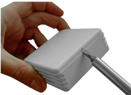
Fig. 3.4.1: Open the cover of the wireless humidity sensor
